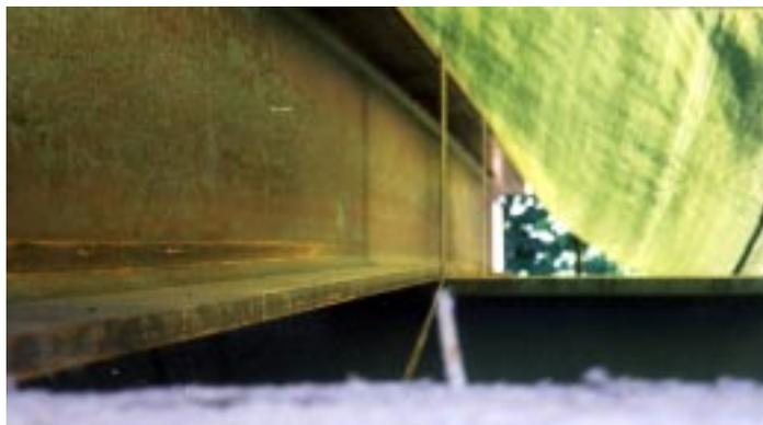
Fig. 84. Deflections in the reaction beams at the end of the loading test on the largest plate.
