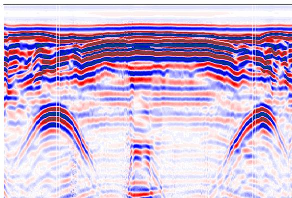
Ground penetrating radar waves can reach depths upto 60 meters in low conductivity materials such as dry sand or granite. Clays, shale and other high conductivity materials may attenuate or absorb GPR signals, greatly decreasing the depth of penetration.
